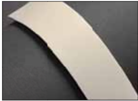
Versico VersiWeld TPO with OctaGuard XT Samples subjected to 275°F heat aging.
